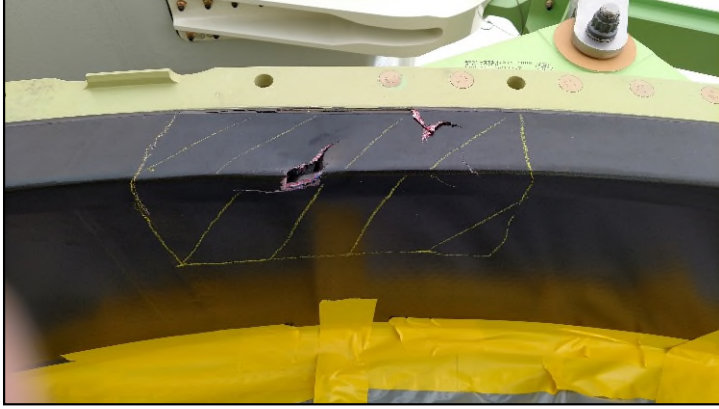
GE90-100 Damaged Trenchfiller
